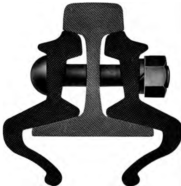
Duquesne Rail Joint
